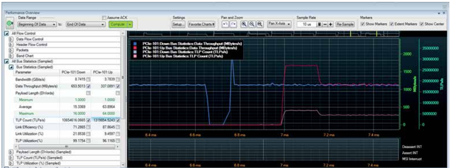
Figure 13. The statistical performance of the link latency, utilization, Flow Control credits, is shown with events such as Interrupts and errors.
