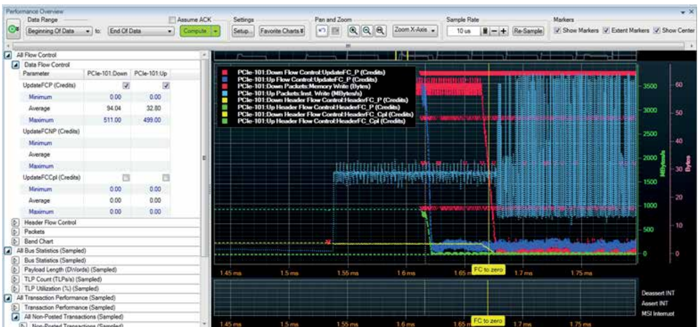
Figure 14. Easily identify credit exhaustion with flow control analysis for data and header flow control analysis.
