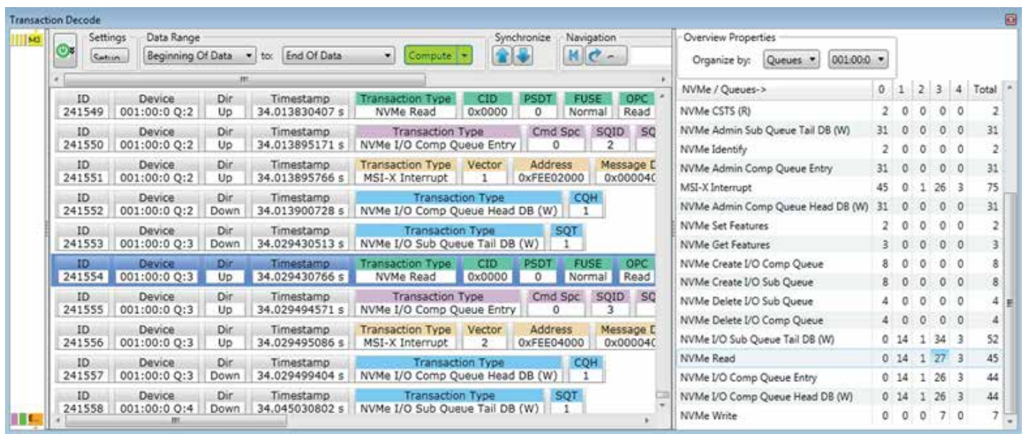
Figure 7. NVMe transaction information provides easy to understand displays of NVMe payloads and PRP messages. Transaction overview of all transactions enables instant access to all messages in the capture trace.
